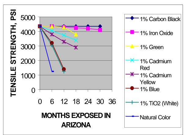
Figure 1: Effect of Pigments on UV stabalization of HDPE PE resins.
