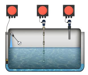
NOTE: The ProAlert® 2 can be used in more than just leak detection applications. It is an excellent high/low level alarm or any other upset condition.
