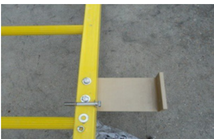
Detail showing cage attachment bracket bolted to ladder railing
