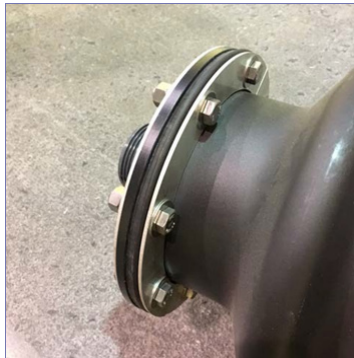
RE-INSTALL GASKET ON BHF THEN INSTALL; 6" GASKET, BLACK PE PLATE, AND 6" SPLIT RING'S USING THE PROVIDED HARDWARE. TIGHTEN NUT ONTO BHF. CONNECT PLUMBING TO FEMALE THREADED BULKHEAD FITTING. HYDRO TEST TANK
