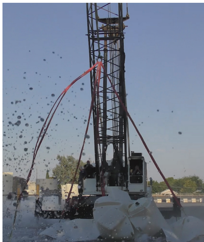
High Density Linear Polyethylene Drop Test Failure
