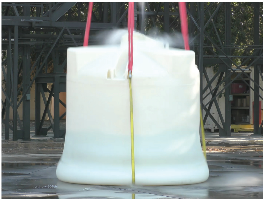
The crosslinked polyethylene tank did not fail or develop any cracks, during the 5 metre drop test.
